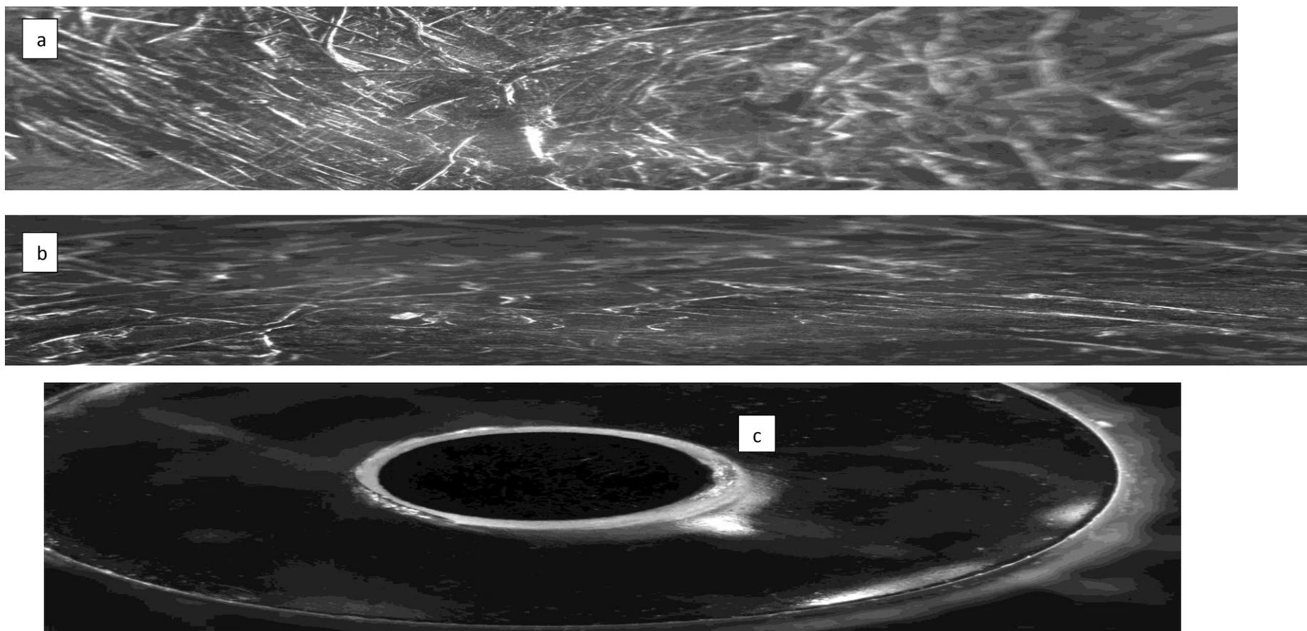
**Figure 4.68: Bismuth electrode surface before (a) and after the electro-analysis (b and c) as viewed under optical microscope**
