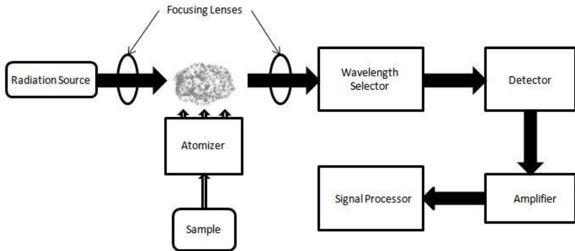
**Figure 2.2: The atomic absorption spectrometer block diagram**
