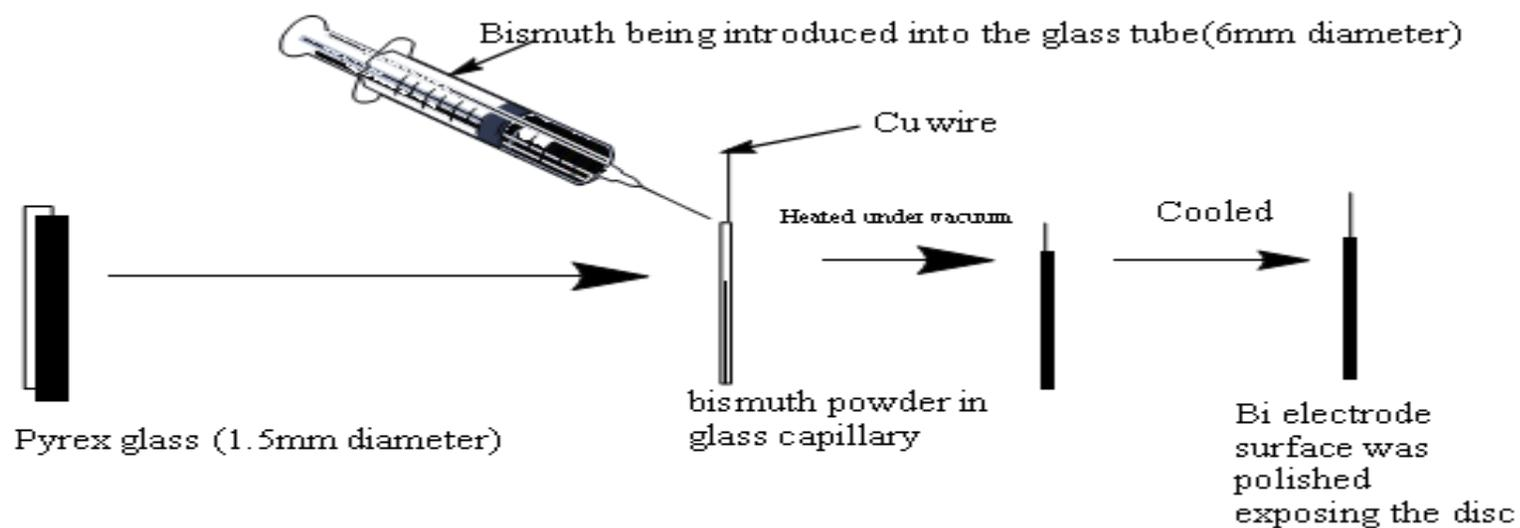
Fig. 3.3 The steps involved in the development of bismuth powder-based electrode
