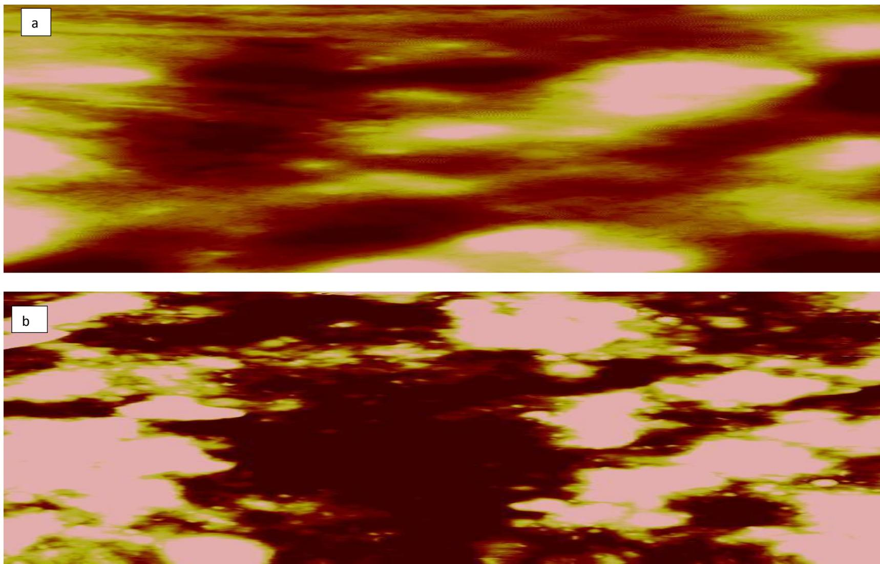
**Figure 4.66: The atomic force microscopic images of bismuth electrode surface before (a) and after (b) the electro-analysis**
