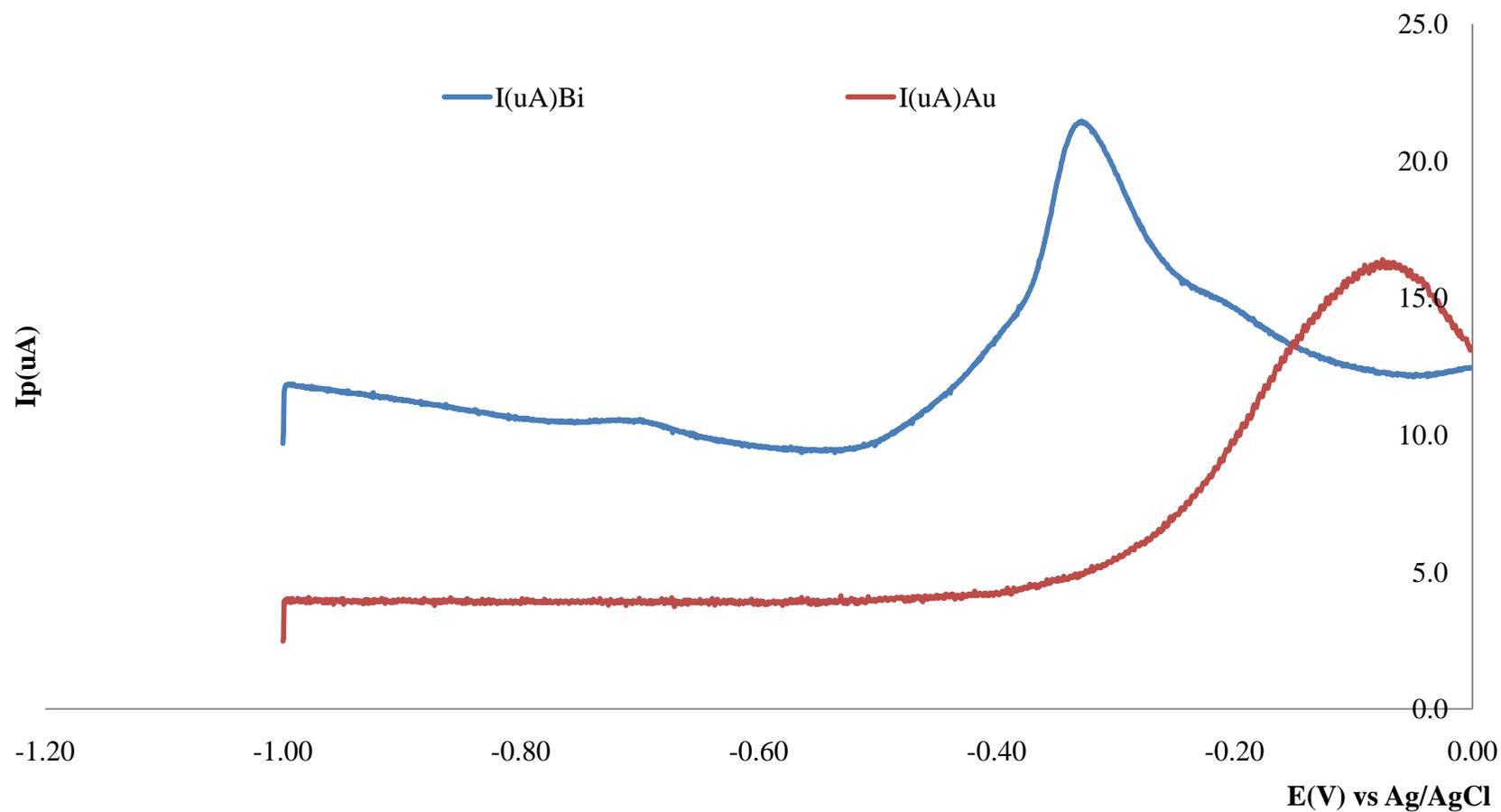
**Figure 4.62: comparative voltammograms of the standard solutions of lead in 100mM NaNO<sub>3</sub> solutions of the supporting electrolytes, the scan parameters where as follows; Estart = -1.0V, Efinal= +1.0V, pulse amplitude = 0.01V, SWV-frequency =80Hz, Estep = 0**
