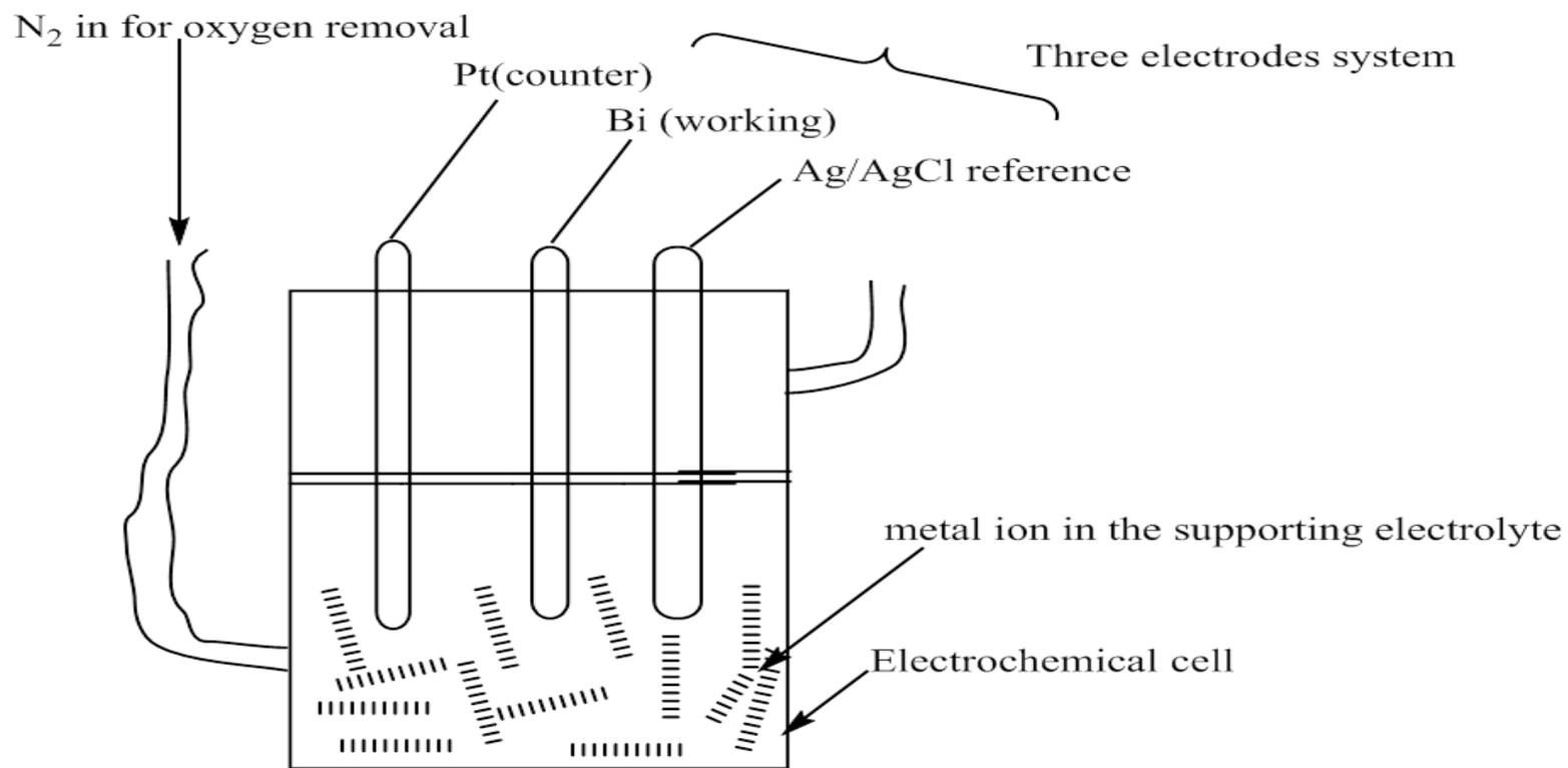
**Fig. 3.4:** Schematic diagram of the three electrode cell used for the electrochemical analysis
