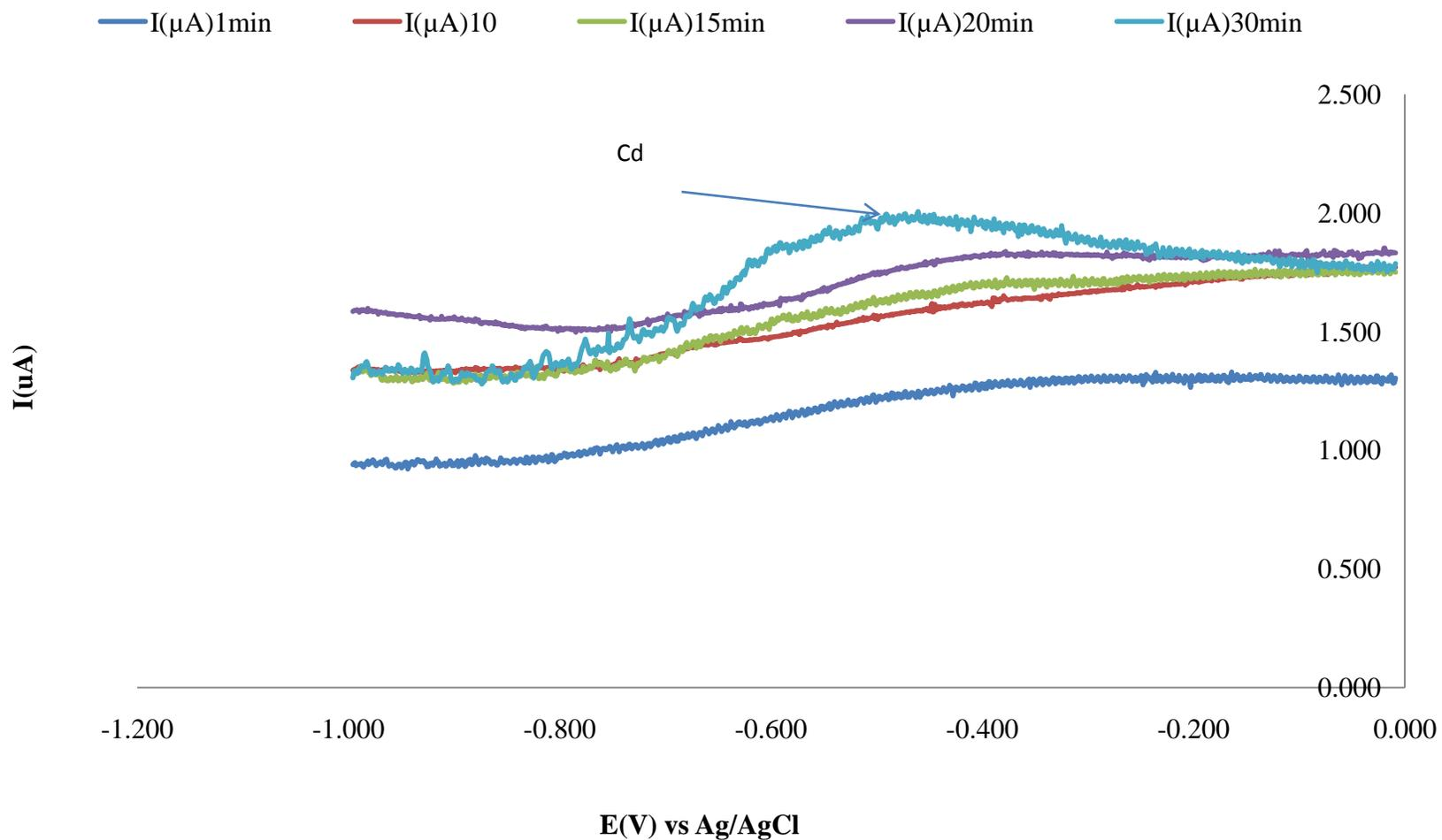
**Figure 4.64: Kinetic studies of cadmium concentrations at different deposition time (1, 10, 15, 20, and 30minutes respectively). Estart = -1.0V, Eend = 0, pulse amaplitude = 0.01V, SQRWV freq = 80V, Estep =0.01V and the current range is 10 $\mu\text{A}$ .**
