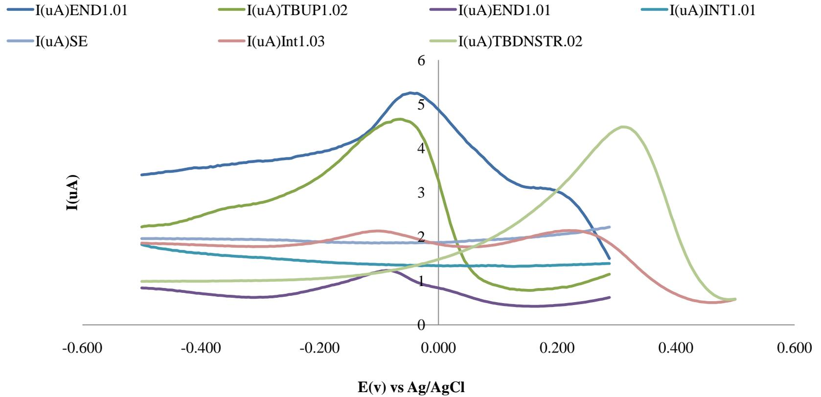
**Figure 4.65:** The SWV voltammograms of the water samples detected using bismuth working electrode, Ag/AgCl reference and platinum counter ; the scan parameters were  $E_{\text{start}} = -0.6\text{v}$ ,  $E_{\text{final}} = +0.6\text{v}$ , swv-frequency = 15hz
