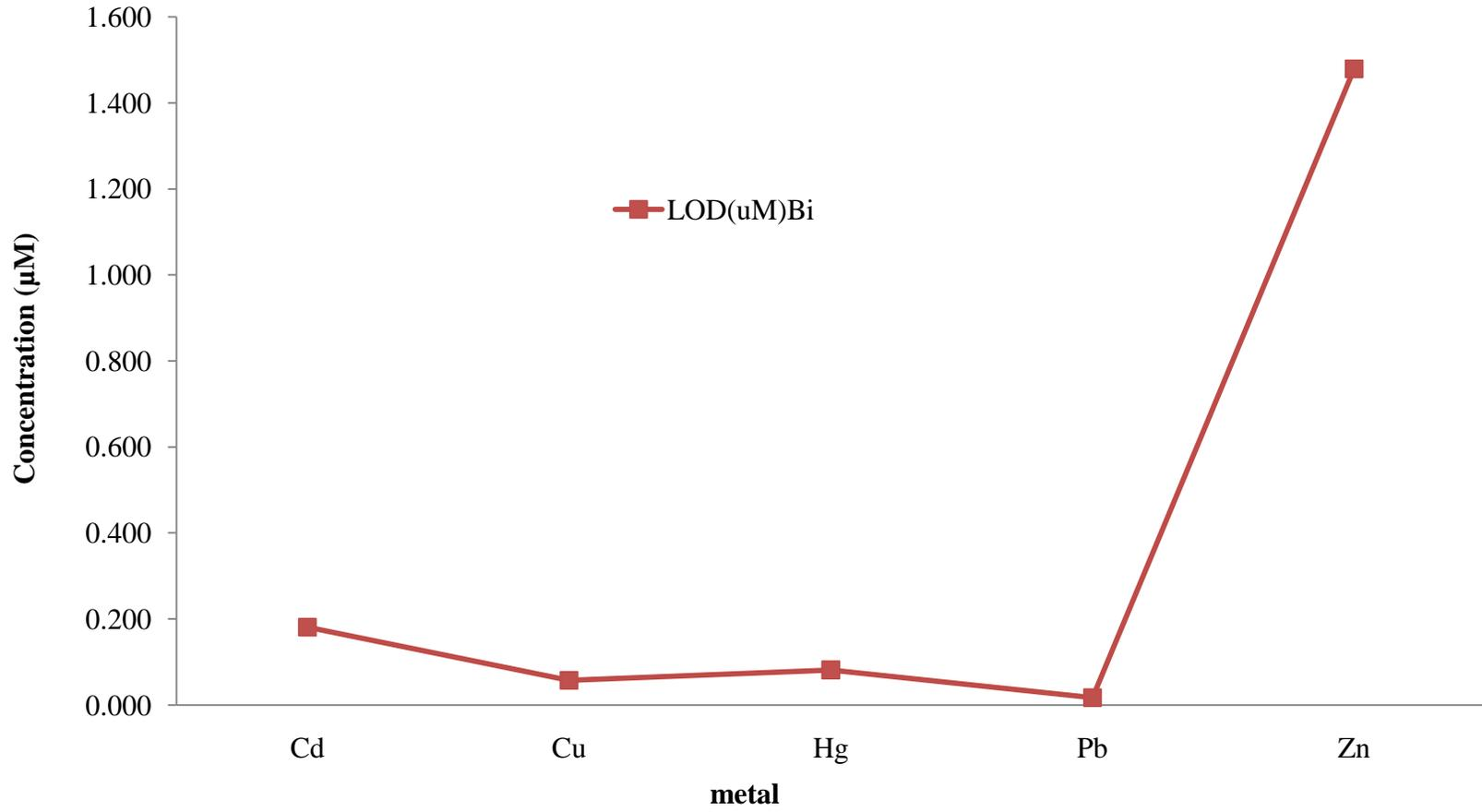
**Figure 4.61: Detection limits of the analysed metals for bismuth (Bi) working electrode**
