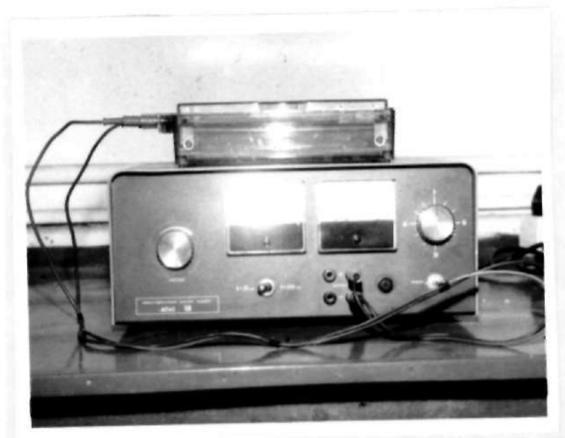
Plate I. Elvi 18 power supply unit and Elvi 70 electrophoresis chamber.
